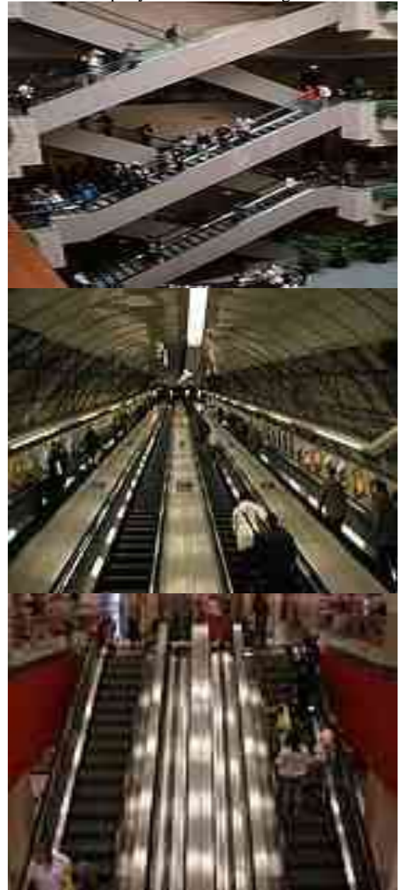
Fig.4 Types of escalator ("Crisscross" "Multiple parallel" "Parallel")
